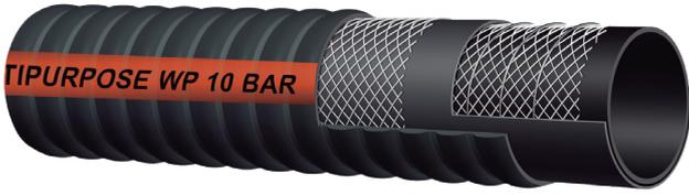
Mandrel hose with corrugated construction and great flexibility. Ideal for suction and propulsion of multiple applications, such as transfer of fuels with a maximum aromatic content of 50% and oils in return line circuits. Due to its flexibility, it is also suitable for wet engine exhaust in boats, where a combination of sea water, diesel moist and engine heat (peaks of 120°C) is required.
